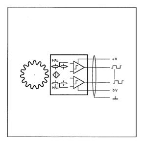
The DSD...W ferrostat sensor is suitable for generating 2 phase shifted speed dependent signals when used with a pole wheel (steel gear wheel, preferably with involute gear form) in order to measure speed and detect the direction of rotation. It exhibits static behaviour with guaranteed pulse generation down to 0 Hz.
