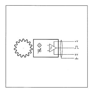
HF speed sensors with amplifier are suitable for generating speed signals from metallic (not necessarily ferrous) pole wheels
