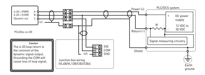
Note: Dynamic ouput must be galvanically isolated when connected to an on time system
