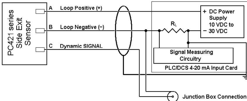
All wire and cable used for installation of the PC421-series sensor should be shielded. Generally accepted instrumentation wiring practice considers the best way to ground the shield is to connect it at the measurement end of the cable. The shield should not be wired to ground at the sensor end of the cable. Wilcoxon R6W, R6GQAI, R6GQI and R6QI type connectors all leave the shield unconnected at the sensor end of the cable.
