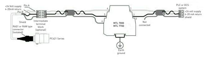
All wire and cable used for installation of the PC421 Series sensor should be shielded. Generally accepted instrumentation wiring practice considers the best way to ground the shield is to connect it at the measurement end of the cable. The shield should not be wired to ground at the sensor end of the cable. Wilcoxon R6W and R6QI type connectors leave the shield unconnected at the sensor end of the cable.
