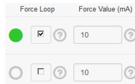
Each loop features a diagnostic test mode that allows the loop current to be forced to any value between 0 mA and 20 mA, without modifying any other settings or mappings. This feature can be used to test the 4-20 mA receiving equipment, loop integrity and maximum resistance compliance. Force mode and mA level are controlled independently for each loop.
