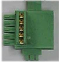
**⚠ WARNING:** The iT300 TBUS is NOT compatible with older iT100/200, iT401 or iT501 series modules. When connecting modules via the TBUS, connect only iT300 series modules together on the same bus. Do not connect any other types of modules or devices to an iT300 TBUS. Doing so may result in damage to the modules.
