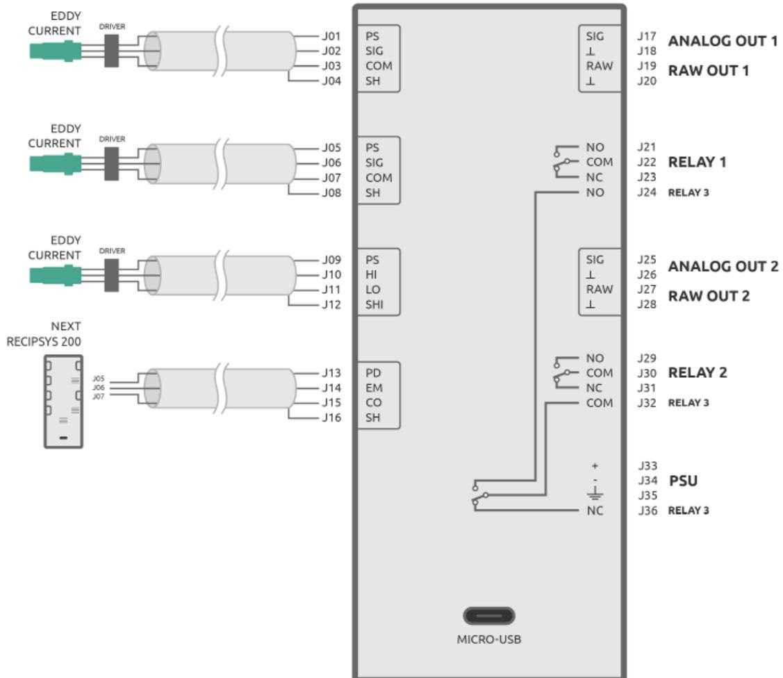
Note: Wiring insulation for relay outputs must be rated at 75°C or higher.
